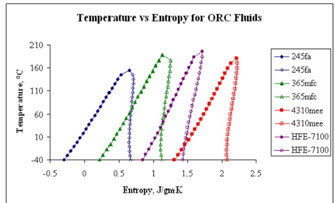
Fig. 5. Temperature-Entropy Domes for Fluorinated Working Fluids
