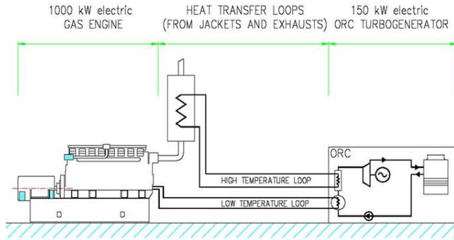
Fig. 4. Biogas ORC Application
