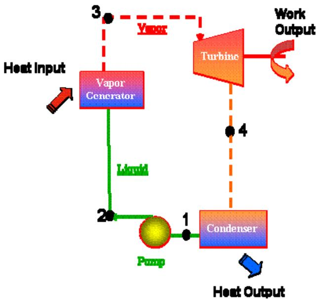
Fig. 2. Simple schematic of ORC system
